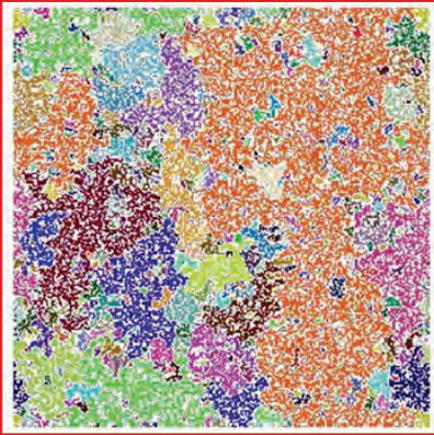
Fig.1: The orange-colored structure is the spanning structure of aluminum on the square lattice at the percolation transition. White denotes holes. The boundary conditions are periodic.
