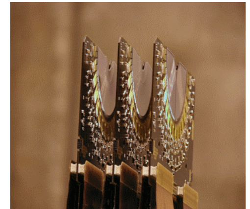
3 bottom halves of VELO modules used in an external “test” particle beam at CERN (top halves are symmetrical)
